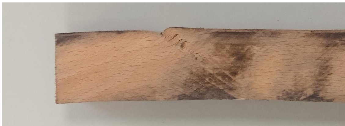
Figure 1: Deep splits along the rays due to pleating in a beech specimen.
