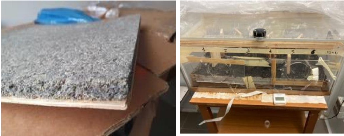
Figure 1: Wood particleboard with encapsulated ethyl palmitate ester as bioPCM processed by the Swedish team for testing the internal bonding (left). A set for testing the susceptibility to mould growth of the bio-composites (right).
