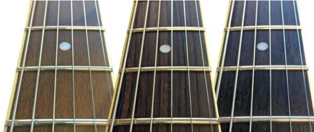
Figure 1: Fingerboards in electrical guitars: modified beech (left), untreated rosewood (middle), modified oak (right).
