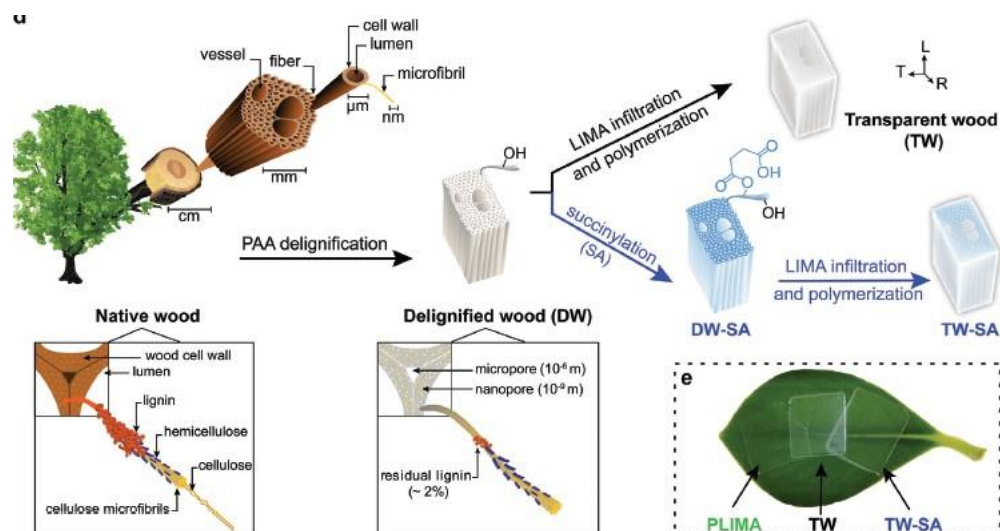
Figure 1: Preparation of fully biobased transparent wood composites. Betula pendula is subjected to peracetic acid (PAA) delignification, then succinylation followed by impregnation by acrylic monomer from limonene oxide and polymerization (Montanari et al. 2021).
